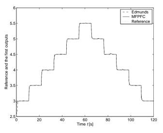
Fig. 6. Comparison of reference tracking for the first output
