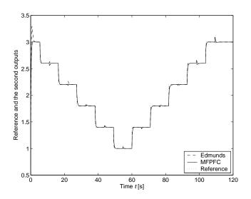
Fig. 7. Comparison of reference tracking for the second output
