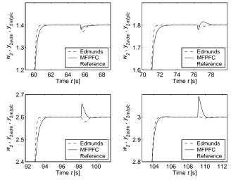
Fig. 11. Transients in tracking of the ascending reference
