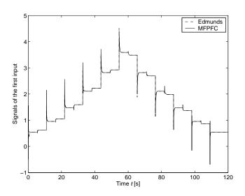
Fig. 8. Comparison of the associated input signals, first input
