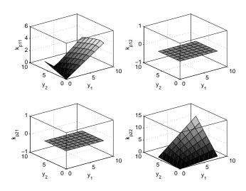
Fig. 4. Parameters of the proportional part of the Edmunds' compensator
